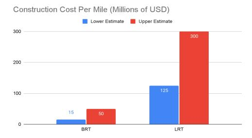
**Figure 2.** Comparison of bus rapid transit and light rail transit per-route-mile construction costs; both ranges are large due to varying road utilization, land value, and grade separation requirements [8,76,82,83].
