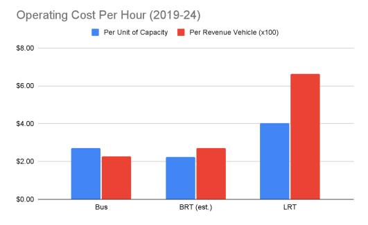
**Figure 3.** Comparison of operating costs per hour normalized per passenger capacity (blue) and vehicle (red, multiplied by 100) [31,56,80].
